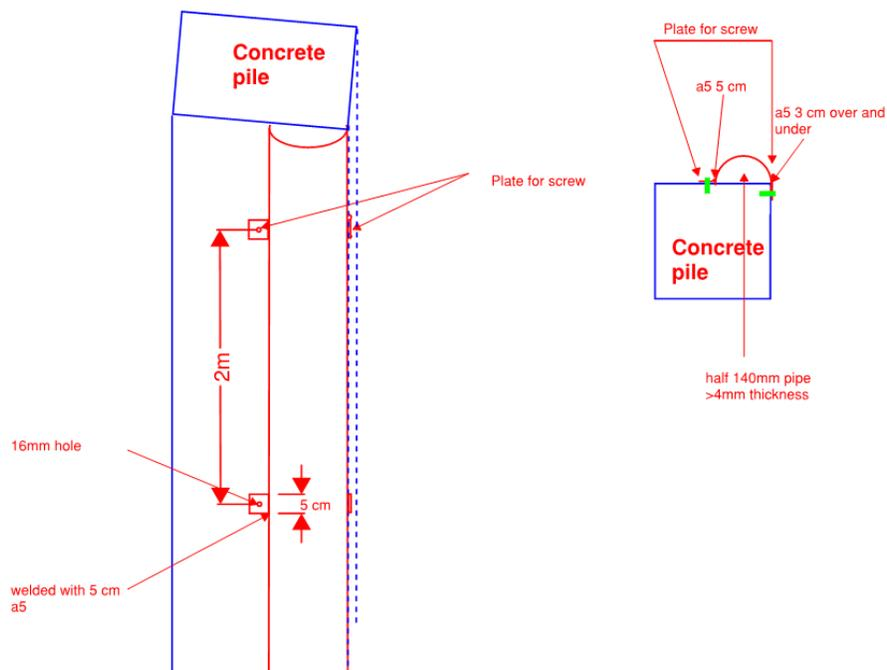
Figure 2: Profile of the pile
