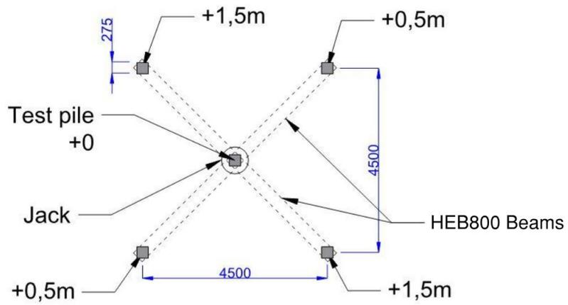
(a) Test setup in 2D plane. Four supporting piles surrounding the test pile
